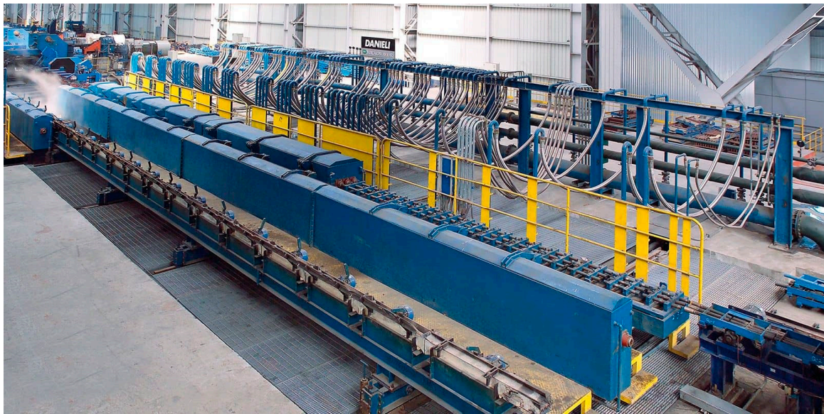
Figure 3. Industrial Tempcore production line.
