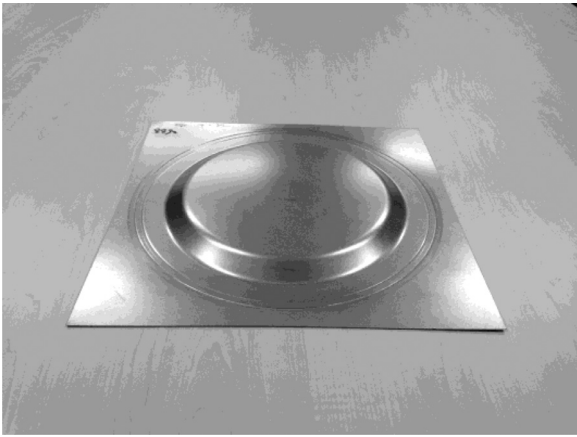
Fig. 11. Dent specimen with a dome height of 12 mm. The dent depth is less than 1 mm and hardly visible in the figure.
