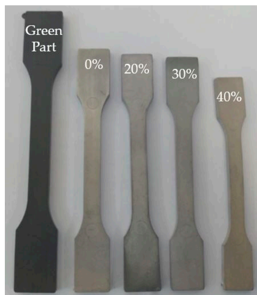
Figure 14. Sintered part and green part for different polymethyl methacrylate (PMMA) volumes.
