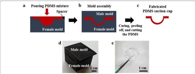
Fig. 1 Fabrication process of the PDMS suction cup, photographs of the 3D printed mold, and fabricated suction cup. **a–c** The PDMS mixture is poured in the 3D printed mold, cured, peeled off from the mold, then cut by a razor blade. **d** 3D printed molds for the PDMS suction cup fabrication. **e** Fabricated PDMS suction cup
