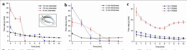
**Fig. 4** Effect of the PDMS suction cup geometry and fabrication conditions on the pumping performance. **a** Effect of diameter (thickness: 1 mm; 12:1 PDMS), **b** thickness (diameter: 10 mm; 12:1 PDMS), and **c** mixing ratio (base/curing agent) of PDMS (diameter: 12 mm; thickness: 1 mm). All measurements are performed in triplicate
