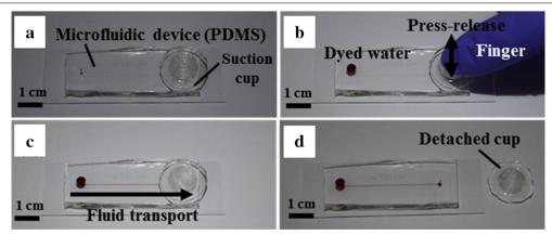
Fig. 3 Suction cup-driven equipment-free fluid pumping. a-d Finger-triggered pumping and reversible integration of the PDMS suction cup to the microfluidic device
