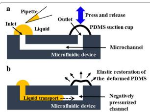
**Fig. 2** Operation mechanism of the PDMS suction cup. **a** A user places the PDMS suction cup at the outlet of the device and presses it to deform, which negatively pressurizes the channel. **b** Liquid is continuously pumped through the channel by the elastic restoration of the deformed PDMS suction cup
