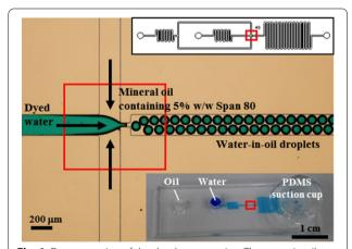
**Fig. 6** Demonstration of the droplet generation. The water-in-oil droplets are continuously generated by pumping the fluids with the PDMS suction cup. The insets show the device geometry and snapshot of the integrated microfluidic device
