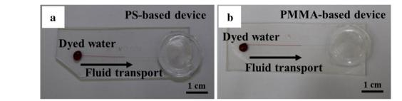
**Fig. 5** Application of the PDMS suction cup for the equipment-free pumping of the thermoplastic-based microfluidic devices. A finger-triggered pumping is successfully performed. **a** Polystyrene (PS)-based device. **b** Poly(methylmethacrylate) (PMMA)-based device
