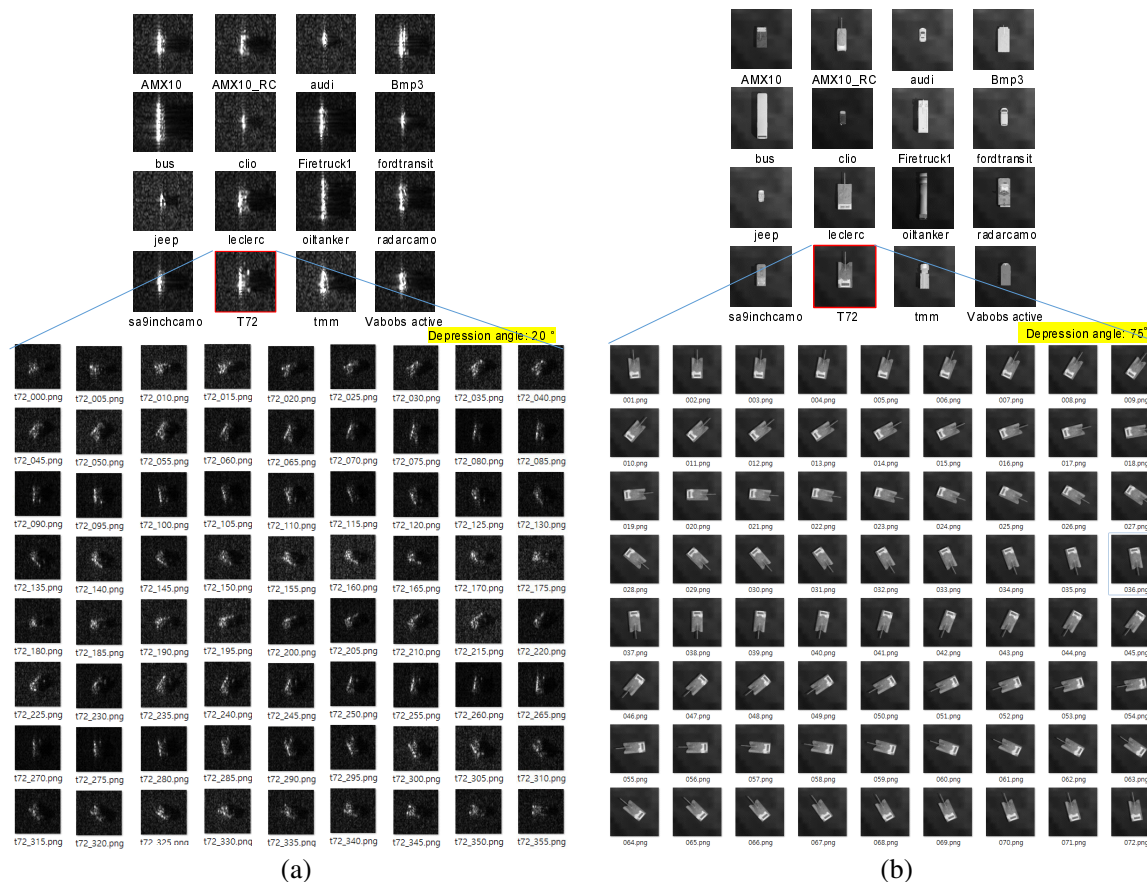
Figure 11. Composition of the SAR-IR target database: (a) 16 SAR targets (top) and 72 aspect views of T72 at the depression angle 20° (bottom); (b) corresponding 16 IR targets (top) and 72 aspect views of T72 at the depression angle 75° (bottom).
