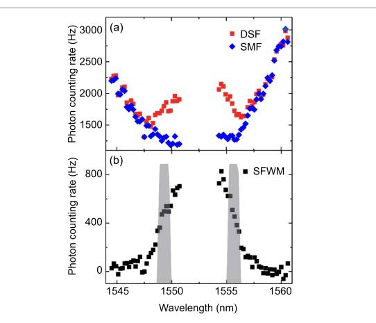
**Figure 3.** Single-photon spectrum measurements. (a) Measured single-photon spectra from a 500 m cooled DSF (red, square) and SMF (blue, diamond) and (b) extracted single-photon spectrum contributed by only the SFWM photons. The gray areas indicate the transmission spectra of filters which are represented by DWDM in insets of (ii) and (iii) of figure 2.
