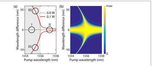
**Figure 1.** (a) Calculated phase matching curve against pump wavelength for a pump peak power of 0 W (black dashed line) and 0.1 W (red solid line) near  $\lambda_{\rm ZGVD}=1555.98$  nm. (b) Normalized probability density spectrum of photon pair emission against pump wavelength for a pump peak power of 0.1 W with a 500 m DSF.
