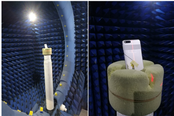
FIGURE 11. Antenna under test in the SATIMO measurement system
